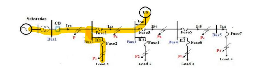
When a fault occurs at another feeder, the operating device located in that faulted feeder should operate. Nevertheless, the fuse at the feeder of the DG may operate and cause unreasonable electricity interruption. As an example; consider the network shown in Figure. The short-circuit fault occurs on position P1. Fuse 2 must operate to remove fault from network, but also Fuse 1 may be tripped because of over-current fed by the DG unit.
