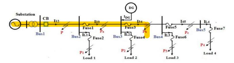
For correct operation of relay it is important that the relay measures the real fault current. As an example, assuming a short circuit at point  $P_b$ , the DG and substation generator contribute to the total fault current ( $I_{Fault} = I_S + I_{DG}$ ), but the relay will only measure the current coming from the substation ( $I_{CB}=I_S$ ). So, the relay detects only a part of the real fault current and may not operate properly.
